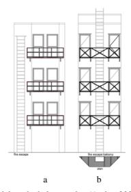
**Figure 15.** (a) Fixed fire escape staircase model on the balcony edge (Andre, 2006; p.144), and (b) Fire escape staircase model connecting between floors through balconies (Andre, 2006; p.133)
