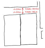
Figure 11. Building height criteria based on the width of the street the facade faces in 1897 Regulation (drawing by authors)
